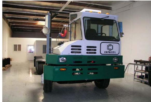
Balqon Corporation was selected to develop and demonstrate the zero-emission class 8 tow tractor. The Balqon Model T324 is an all-electric terminal tractor with a payload capacity of 60,000 lbs and an estimated range of 40 miles on a single charge. The vehicle is equipped with a fast charge capability that allows the vehicle to be fully recharged in 30 to 45 minutes.
