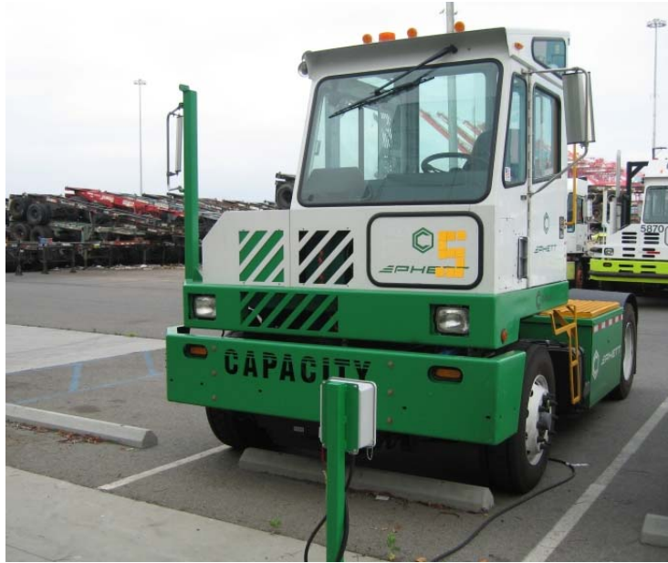
Figure 1. PHETT™ at Pier T charging stall
