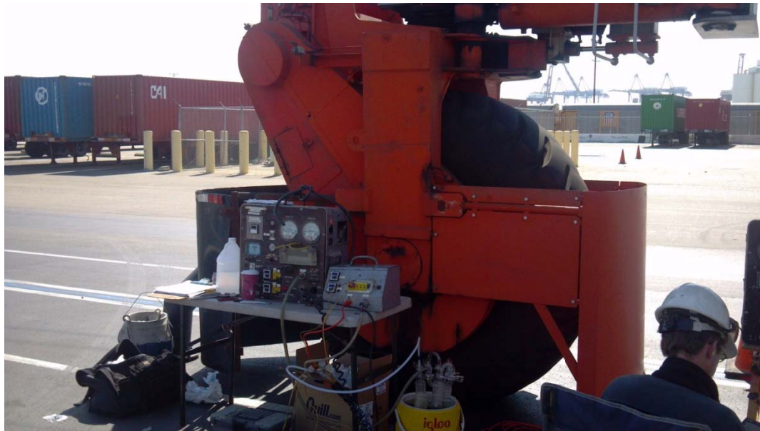
Photo 3: Emission samples being gathered and measured by Best Environmental
